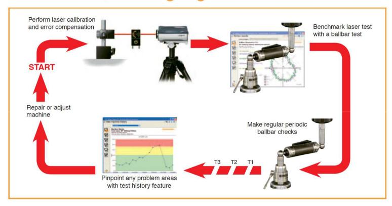
The Renishaw ballbar system is internationally recognised as the ideal solution to quickly check machine tool performance and benchmark in between scheduled laser calibrations.
