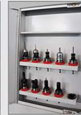
▲ 增加刀倉設計 Second tool magazine located in front of the machine
