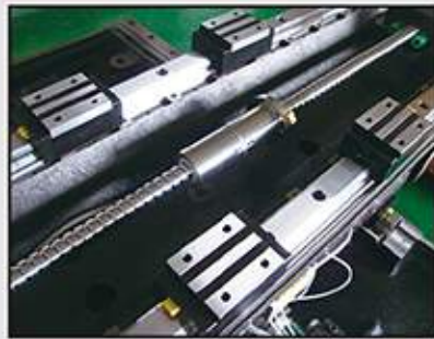
▲ 精密滾珠線性滑軌 Precision ball linear guide ▲ 精密高剛性滾柱線性滑軌 Precision roller linear guide ▲ 精密斜角滾珠軸承 Precision angle bearing ▲ 精密雙螺帽滾珠螺桿 Precision ballscrew
