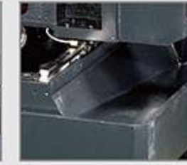
▲ 底座大斜度排屑設計 Steep slope surface on the base for chip removal
