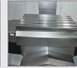
▲ 伸縮防屑蓋斜度設計 Slope on telescopic cover for easy chip flow
